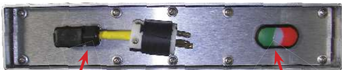
Water Tight Electrical Plug
